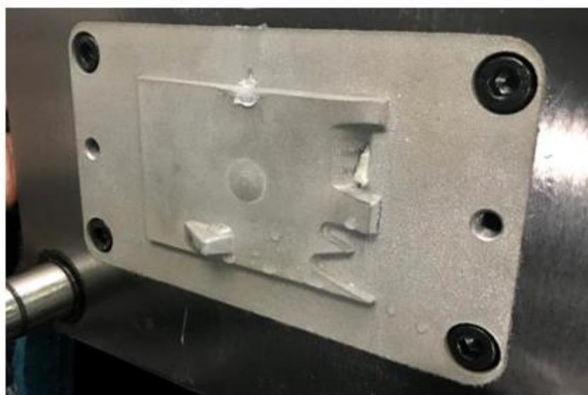
**Figure 2. Example of a rapid tooling insert produced through AM in a modular mould base**
